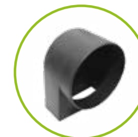
Odour trap for sump unit for retrofitting DN 100/150 Installation: Insert the odour trap from the inside and connect with the sewage pipe.
