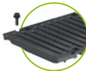
ductile iron slotted grating SW 16 /300, class D, F 4-point bolted
