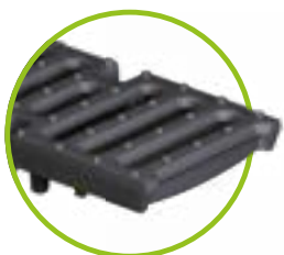
Ductile iron slotted grating SW 14/100, 14/150, 14/200 for NW 100 to 200 class E, with fiX-locking for NW 100 to 200 Class D, F 4x bolted
