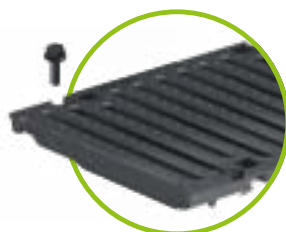
Ductile iron slotted grating SW 16 /300, class D 4-point bolted
