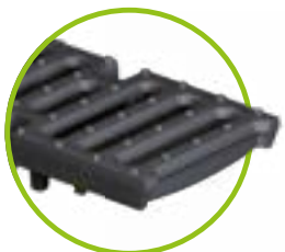
Ductile iron slotted grating SW 14/100, 14/150, 14/200 For NW 100 bis 200 class E with fiX-locking for NW 150 to 200 Class D 4-point bolted
